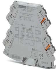
Two-channel output loop-powered 2-way repeater power supply with plug-in connection technology for the electrical isolation of analog signals. Input signal = output signal: 0(4) mA ... 20 mA. Screw connection technology.
